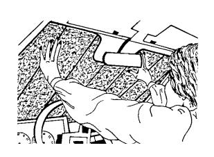
Pull down each sun visor to hold the Sunshade in place. There is nothing to attach to your vehicle. The Sunshade is not designed to fit tightly against the windshield.
