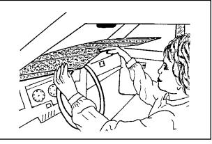
With both hands, lift the top of the Sunshade into the windshield area. (Be sure not to bend corners while installing, or damage to the inner insulator may occur.) On Eyesight equipped vehicles, do not allow the Sunshade to contact the Eyesight housing or
